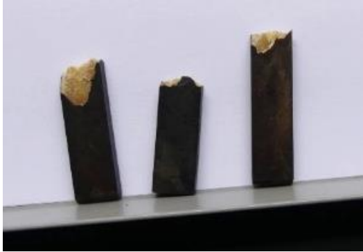
Embrittled and strongly discolored test specimens of PPA (6T/6) GF35 after storage in coolant (water / glycol) for 1,000 h / 150 °C.
