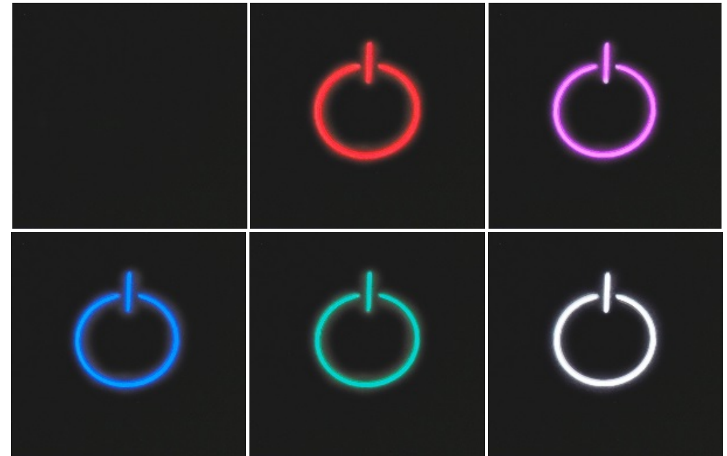
Pictures: Alcom LDDC backlit with symbol template on the Alcom Lighting Demonstrator Top left: Light switched off, other pictures: illuminated with RGB LEDs
